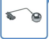
Direct mechanical lever operated Float valves, single or double ported in C.I., C.S., and SS Constructions Operating mechanism is specially designed to be mounted on all types of tank equipment and serves the purpose of a liquid level controller or drain.
